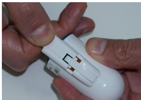
Figure 23 – New Finger probe connection
